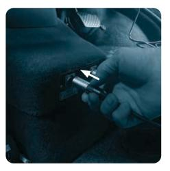
Figure 2-15 SRS side airbag plug & wall socket
