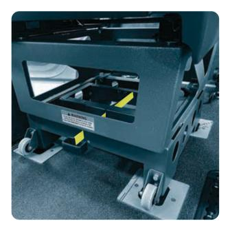
Figure 2-10 Removable Seat Unlocked
