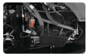
7.5A & 40A fuses in engine bay near battery
