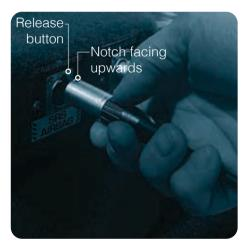
Figure 2-14 SRS side airbag plug & socket
